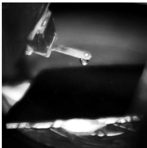
Fig. 1. Beryllium bronze cantilever mounted on NT-206 SPM
